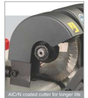
AlCrN coated cutter for longer life
